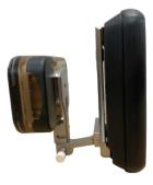
Attach sensor to bracket
