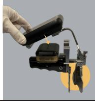
Note Lantern IMU measures rotation of navigation unit in response to the angle of the femoral paddle
