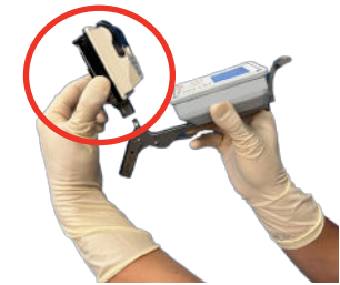
1D. Depress lever to attach sensor to bracket, matching arrow to arrow.
