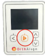
1B. Press orange "home" button to turn on navigation unit.
